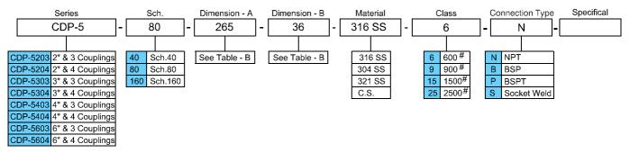
These are the standard ordering number, PMT will provide the final ordering number based on the customer's specification.
